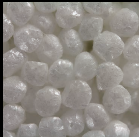
▲ If no one else will give an element a home, the lighting industry steps up. This lutetium bromide is lovingly created to the highest standards of purity for use in high-intensity discharge lights.
