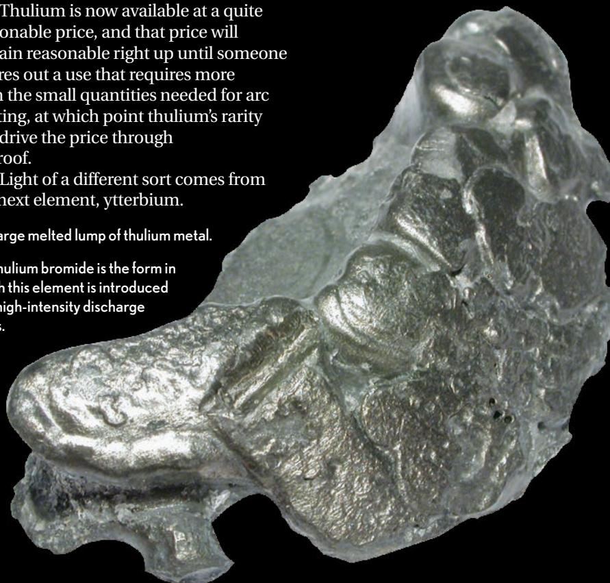
▲ Thulium contributes a critical broad range of green emission lines to metal halide lamps.
