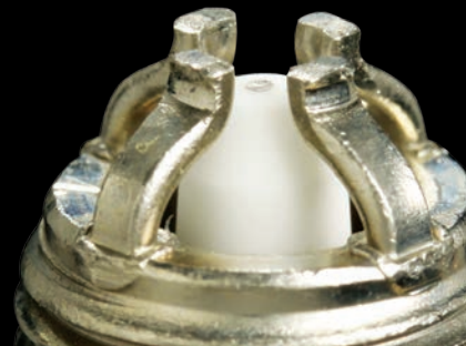
▶ Platinum spark plugs are now quite common and last nearly the life of a car.
